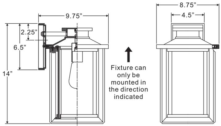
Fixture can only be mounted in the direction indicated
